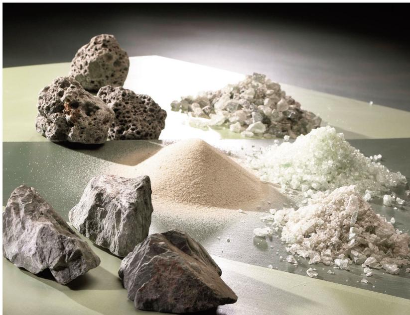
Fiber glass, rock wool and slag wool are made from a combination of natural and recycled ingredients such as basaltic rock, blast furnace slag, recycled glass cullet and sand. The natural ingredients, sand and rock, are readily available. The use of blast furnace slag and glass cullet are recycled materials that are transformed into a product that saves energy and reduces pollution.
