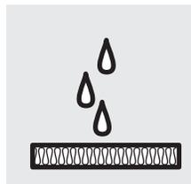
up and hold water, thus it resists permanent loss of R-value. Because it is inorganic, it is naturally fire resistant. If fiber glass insulation becomes saturated as the result of flooding or other catastrophic events, the manufacturer of the product should be consulted to determine whether the product should be replaced.
