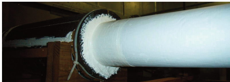
Figure 2. Pipe -Insulation Specimen Installed on a PIT. Vapor Retarder Mastic is used to seal the 6" Insulation Transition Sections to the Thermal Guard
