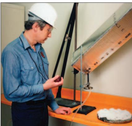
Air ducts should not continue to burn progressively, and exterior surfaces of the material should not drop particles that are capable of igniting combustible materials such as cotton.
