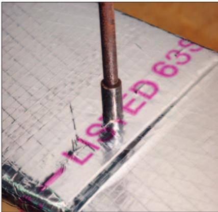
During fabrication and installation, unintentional mishaps such as a dropped tool can occur and the duct must be able to withstand them. Even in routine service, air ducts may encounter abuse. This test indicates just how well the duct will resist damage during and after installation.
