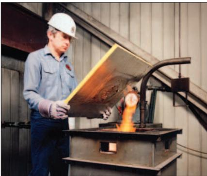
Test Procedure: The exterior surface of the fibrous glass duct material is subjected to a gas flame from a furnace. It must resist penetration of the test flame for 30 minutes while supporting a concentrated load of 2 pounds per square inch.
