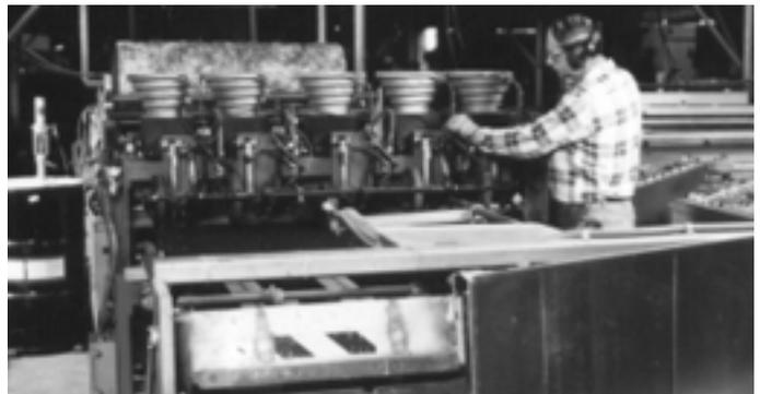
*Fig. II-2. Cutting and processing fibrous glass duct liner on an automatic coil line.*
