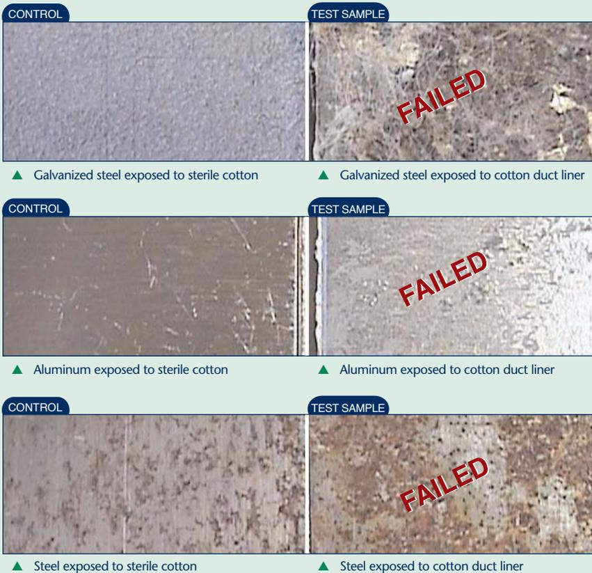
NOTE: Copper was also tested, but showed no corrosion. Copper is rarely in contact with duct liner materials.
